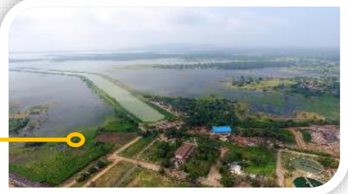
5.5 Km Long Dedicated Water Intake Channel from Hirakud Reservoir, with Contracted allocation 1.3 L m3/day
